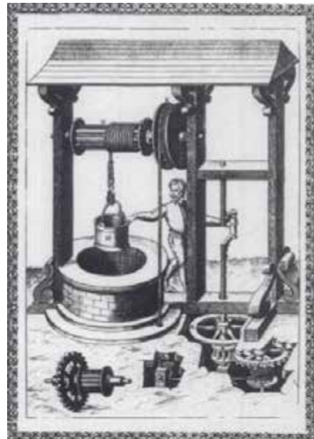
意大利工程师阿戈斯蒂诺·拉梅利 (Agostino Ramelli) 著作中使用绞盘打水的水井 (windlass well), 1588 年出版 The windlass well described in the work of Agostino Ramelli, an Italian engineer, published in 1588
